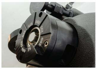
Warning: The pressure relief valve must be properly set prior to operation.
